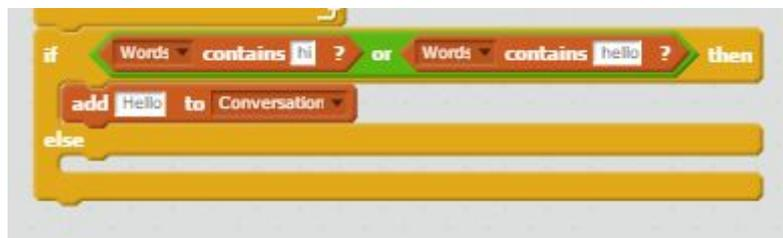
Give it a test. On entering the word 'Hi' into the input box we should get a response of 'Hello' back from our chatbot.
